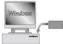
Windows computer (requires SCSI adapter) SCSI adapters must be configured for your system. See the information provided with your SCSI adapter
